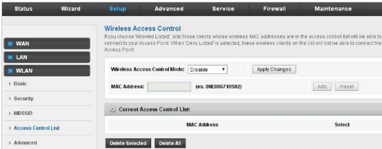
Figure 5-29 Wireless Access Control
