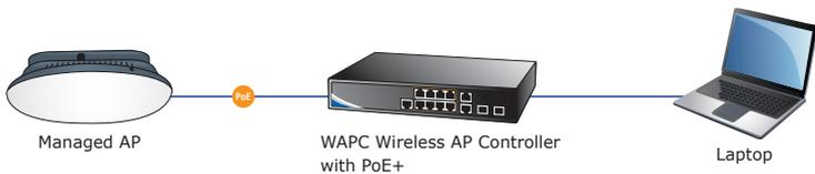
Figure 4-1 Topology of AP Controller Connection
