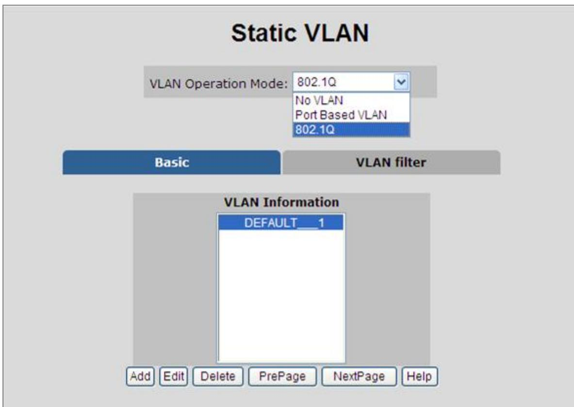
Figure 4-4-2-1: Static VLAN interface
