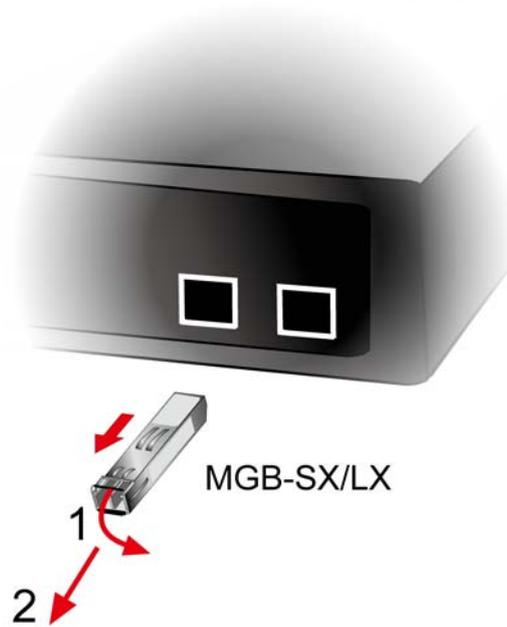
**Figure 2-1-8** How to Pull Out the SFP Transceiver
