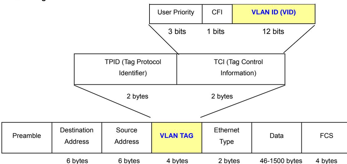
The Ether Type and VLAN ID are inserted after the MAC source address, but before the original Ether Type/Length or Logical Link Control. Because the packet is now a bit longer than it was originally, the Cyclic Redundancy Check (CRC) must be recalculated.
