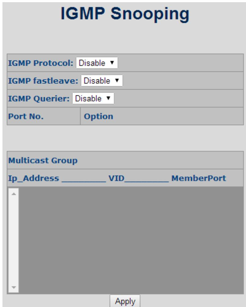
Figure 4-7-2-1: IGMP Configuration Interface Screenshot
