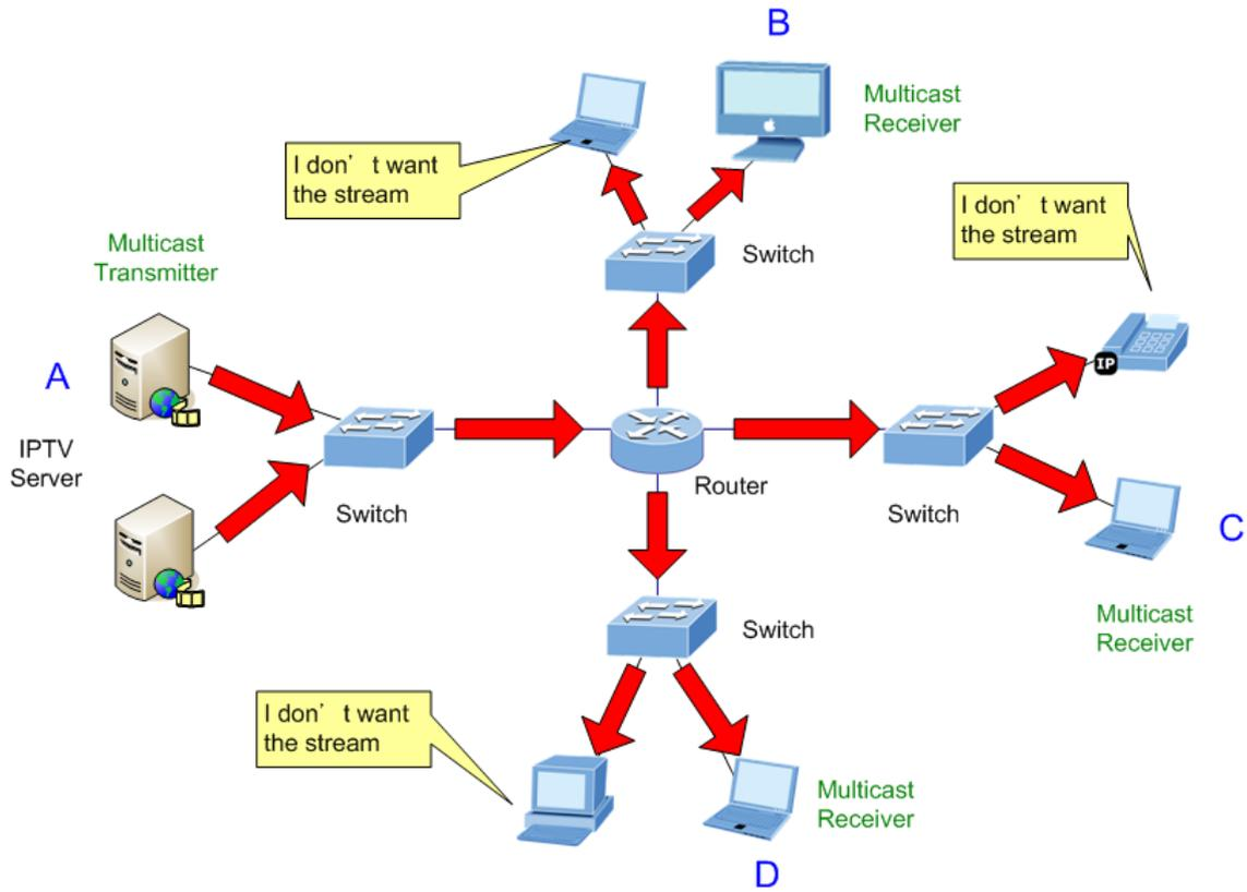
Figure 4-7-1-2: Multicast Flooding
