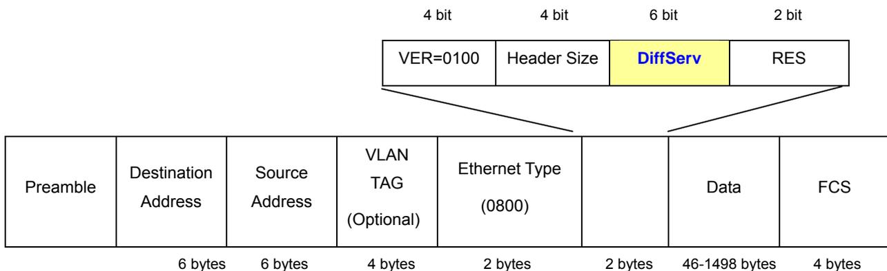
Figure 4-15-4: IPv4 Frame Format
