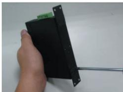
**Step 3:** Use the screws to screw the wall-mount plate on the Industrial Power over Ethernet Extender.
