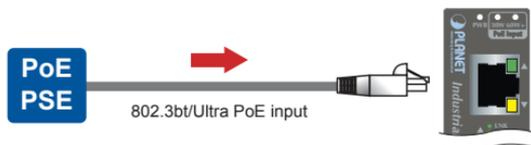
**Step 2:** The PSE delivers both Ethernet Data and PoE power over UTP cable to the IPOE-E174 and the **“PoE IN”** LED will be lit steadily.
