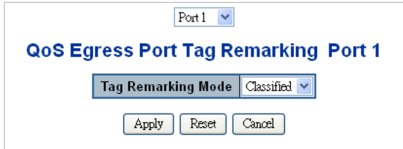
Figure 4-9-7: QoS Egress Port Tag Remarking Page Screenshot
