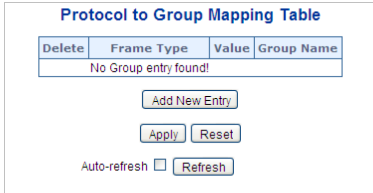
Figure 4-6-21: Protocol to Group Mapping Table Page Screenshot
