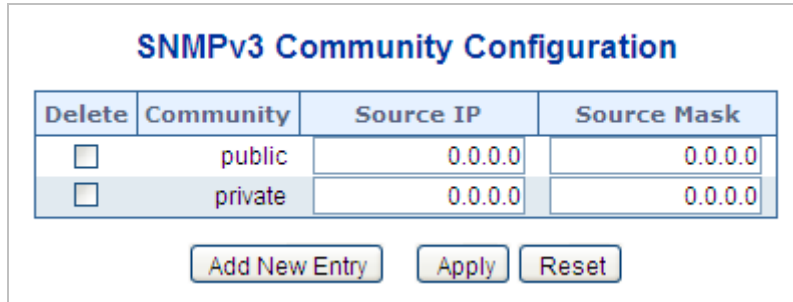
Figure 4-3-4: SNMPv3 Communities Configuration Page Screenshot
