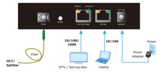
Figure 3-1: EPN-103 connection diagram
