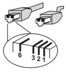
The standard RJ-45 receptacle/connector
