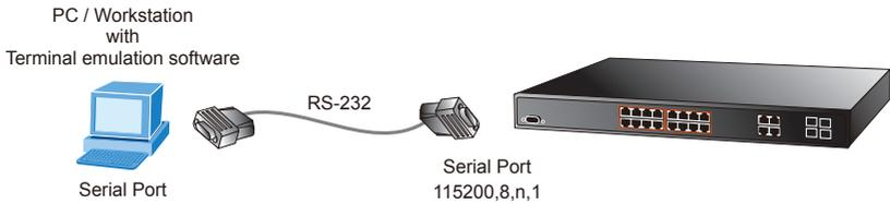
A terminal program is required to make the software connection to the Managed Switch. Windows' **Hyper Terminal** program may be a good choice. The Hyper Terminal can be accessed from the **Start** menu.
