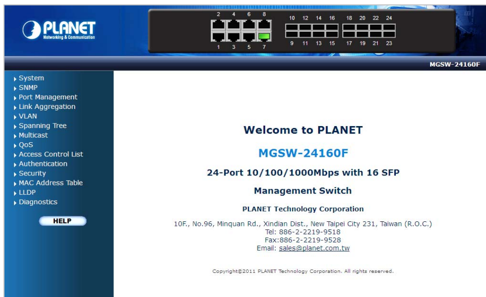
Figure 3-4 Web Main Screen of Managed Switch
