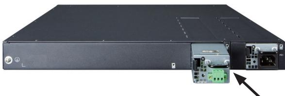
Figure 3-2 Inserting the XGS3-PWR150-48
