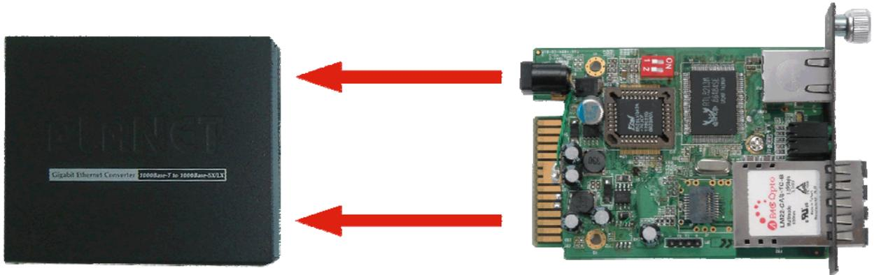
Step 2- Remove a blank faceplate from an empty expansion slot on the front of the chassis. The GST-80x Media Converter board can be installed in any expansion slot.
