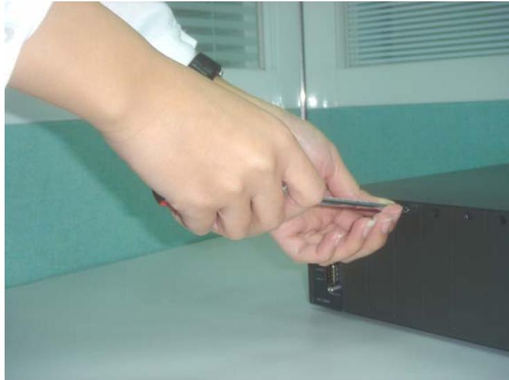
Step 3- Slide the GST-80x Media Converter board into the expansion slot, aligning it with the guide rails, until it firmly connects to the chassis' backplane.
