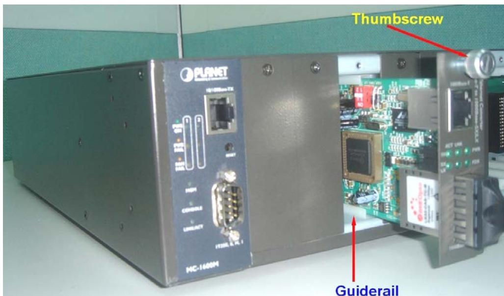
Step 4- Secure the GST-80x Media Converter board to the chassis by tightening the thumbscrew.
