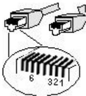
The standard RJ-45 receptacle/connector
