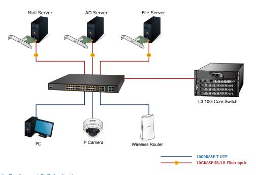
Layer 2+ VLAN Static Routing and PoE Application
