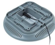
**Step 4:** Attach the WNAP-C3220A to the mounting bracket.
