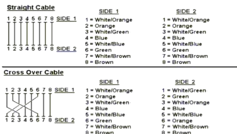
Figure A-1: Straight-Through and Crossover Cable
