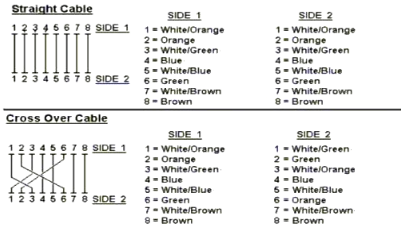
Figure A-1: Straight-Through and Crossover Cable
